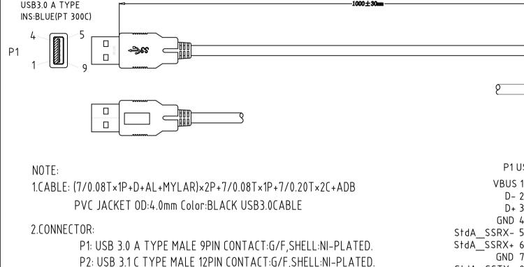
P1 USB3.0 AM P2 USB3.1 C -A4.B4.A9.B9 VBUS 1 -White A7 Green A6 Black A1,B1,A12,B12 GND 4 Orange A3 StdA SSRX-5 Purple A2 StdA SSRX+ 6 GND 7 -◆ 地线 Drain -A1.B1.A12.B12 Blue B10 StdA SSTX-8-Yellow B11 StdA SSTX+ 9 Shield SHELL
